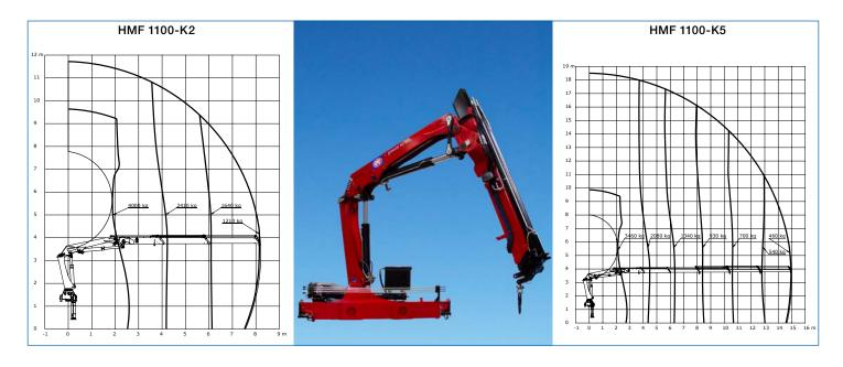
The HMF 1100-K model with dual Power Plus link arm system and manual ground control or stand-up controls and fixed flow pump.
